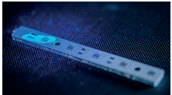
Fluorescing flux residues on a printed circuit board detected through an imaging process.
