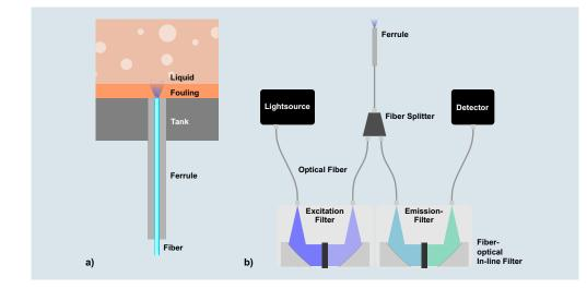
a) F-Fiber installed in a production system. The fouled surface inside the vessel is excited by UV light.
