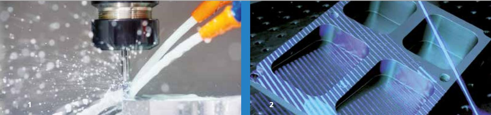
1+2 A fluorescence imaging measurement system by Fraunhofer IPM detects contamination or defects on surfaces directly in the production line.
