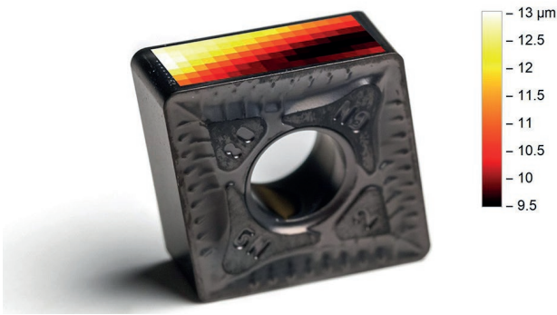
LIBS imaging shows that the coating thickness varies locally on an indexable insert, with values ranging from 9.5 to 13 µm.
