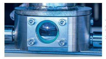
LiVision uses a short pulse laser to convert a tiny amount of liquid into plasma. The plasma flash provides valuable elemental information, particularly the lithium content.
