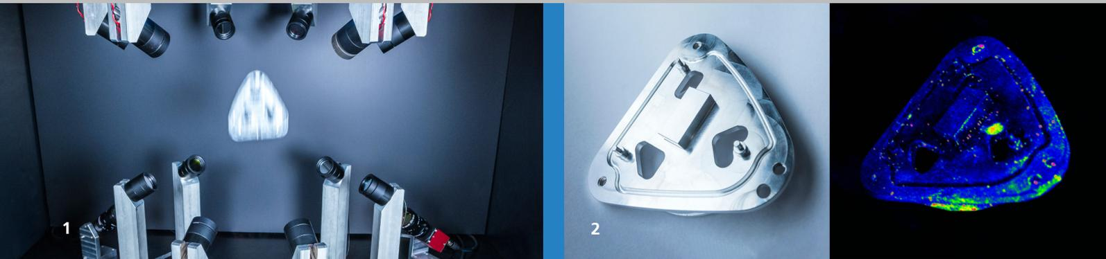
1 The F-360° inspection system records objects from different directions in free fall using several cameras. This is how 100 percent of the object surface is captured in a single recording process.
