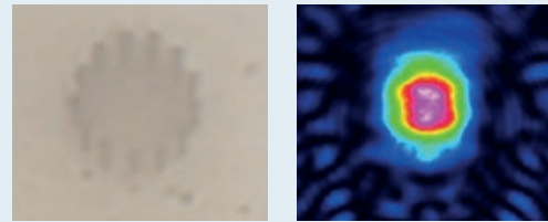
Left: Endfacet of a laser-inscribed waveguiding structure Right: Typical mode profile
