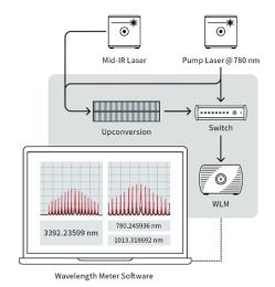
Schematic view of a waveguide-based upconverter module, integrated in an "upconversion wavemeter" setup. This setup was developed in the Project NeW-VIEUW (see left). Through difference frequency generation, the mid-IR light is converted into the near infrared, where the wavelength is measured with a near infrared wavemeter.
