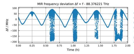
Frequency measurement of a free running 3.392 µm HeNe laser using the "Upconversion wavemeter" (see **Project New-VIEUW**). The instantaneous frequency is given as the difference against 88.376221 THz.
