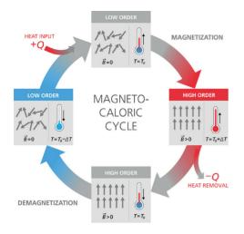
**Magnetization** Magnetocaloric (MC) material is exposed to a magnetic field and heats up due to the generated magnetic order from temperature  $T_0$  to  $T_0+\Delta T$ .
