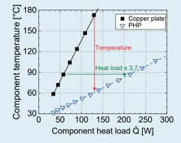
PHP are characterized by high heat transfer capacity and low thermal resistance. Placed on a PHP (here 100 x 50 x 2.5 mm<sup>3</sup>, 21 °C cold side temperature), a hot component reaches a much lower temperature (blue data points) than on a copper plate of the same size (black data points). A critical temperature of typically around 80–90 °C is only reached at three to four times higher heat loads.
