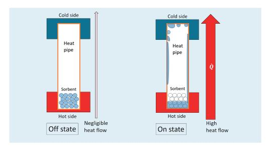
Thermal switches with temperature-dependent regulation using sorbents.
