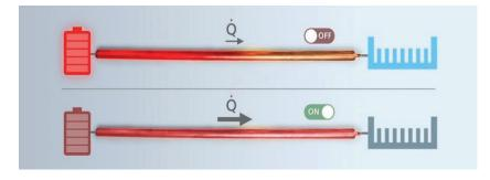
Switchable heat pipes are compact and do not require any moving parts. They are easy to integrate and guarantee a very high heat transport capacity.
