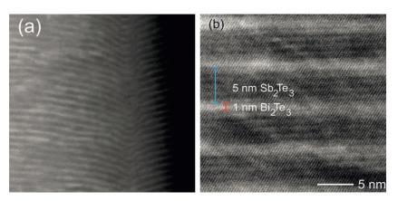
Superlattice layered stacks made of the thermoelectric materials  $Bi_2Te_3$  /  $Sb_2Te_3$ . TDTR measurements have proven that these nanoscale superlattices are capable of significantly reducing thermal conductivity in comparison to homogeneous materials.
