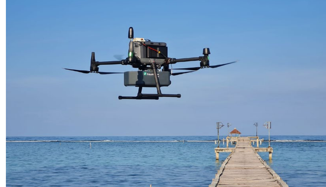
The Airborne Bathymetric Laser Scanner flies over the coastal region of Pramuka.
