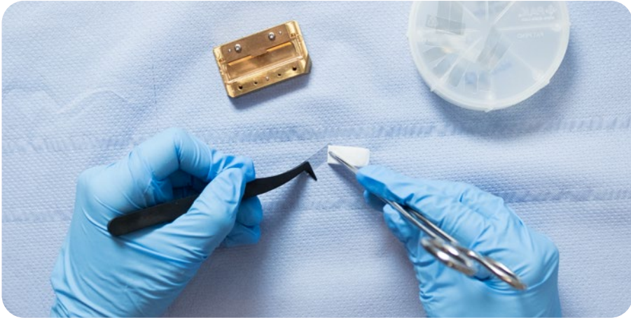
I am holding a periodically poled lithium niobate (PPLN) crystal in chip format with my tweezers. First, I thoroughly clean its surfaces with a lens-cleaning cloth.
