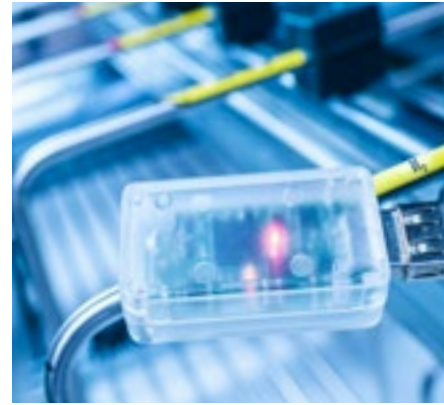
Small and sparing: The H 2 sensor, which measures just 6×2 cm 2 and can be connected to a computer, measures H 2 concentrations of 0.4 percent and above in air in under a minute.
