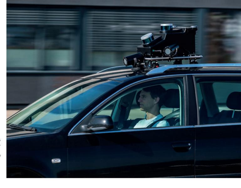
through the city. All measurement data is automatically anonymized before being stored locally and then immediately transmitted to a geographic information system via the 5G network. Al-based algorithms semantically enrich the data streams and create the necessary data models for the digital twin.
