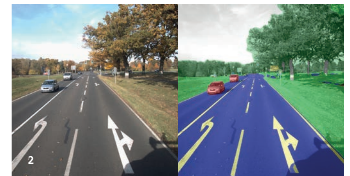
1 Recognizing, classifying and locating objects on the roads is time consuming. Pattern recognition using artificial neural networks automates this process.
