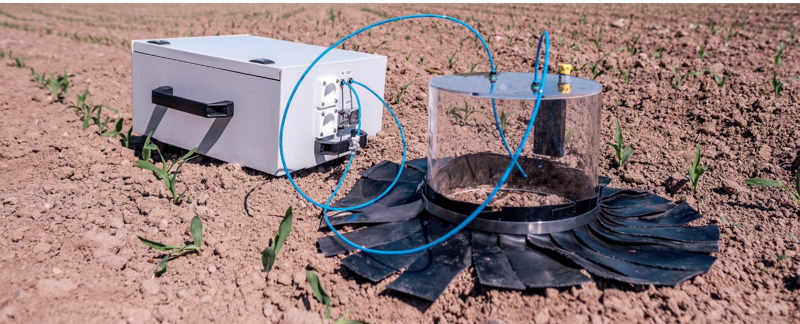
Mobile nitrous oxide sensor: The sample is taken at ground level using a bell jar; the actual measurement system is concealed in a case.
