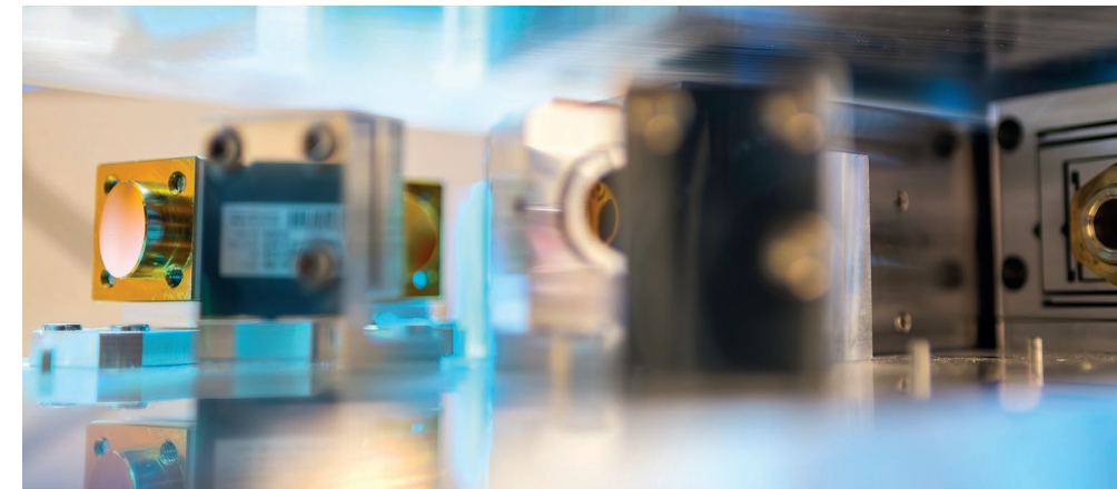
Using an innovative measurement concept that employs interband cascade lasers (ICL) as the light source, nitrous oxide can be measured in the mid-infrared range unimpeded by cross-sensitivity with other gases. The entire process is extremely quick and can be performed out in the field.
