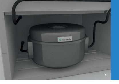
**1+2** CAD model of a magnetocaloric cooling system. A rotating permanent magnet generates a magnetic field that heats and cools the seriesconnected magnetocaloric segments.
