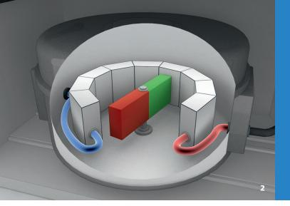
heat transfer through the evaporation and condensation of a fluid in a hermetically sealed volume. Such heat exchangers, also known as thermosiphons, are used as solar collectors or in computer cooling. The heat pipe concept is an innovative method for implementing a magnetocaloric cooling cycle.
