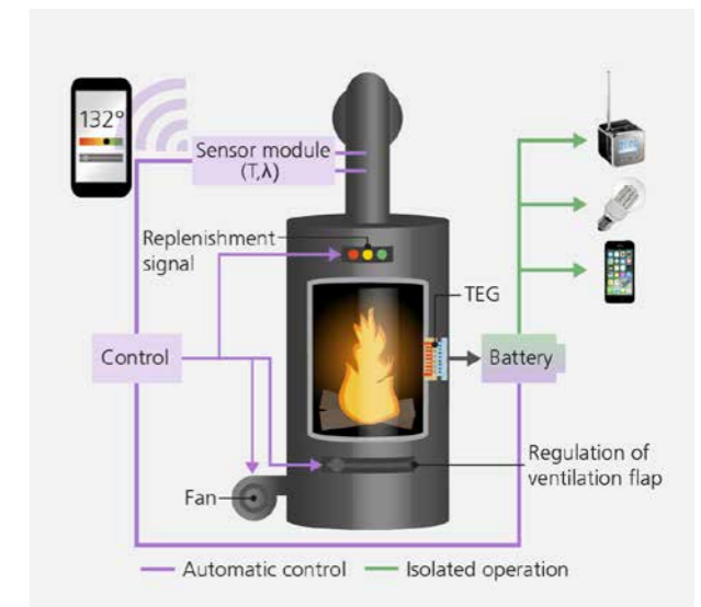
Fitting small furnaces with a thermoelectric high-temperature generator will in future provide enough electric power for small regulators that signal the right time to add more logs or optimize air intake.
