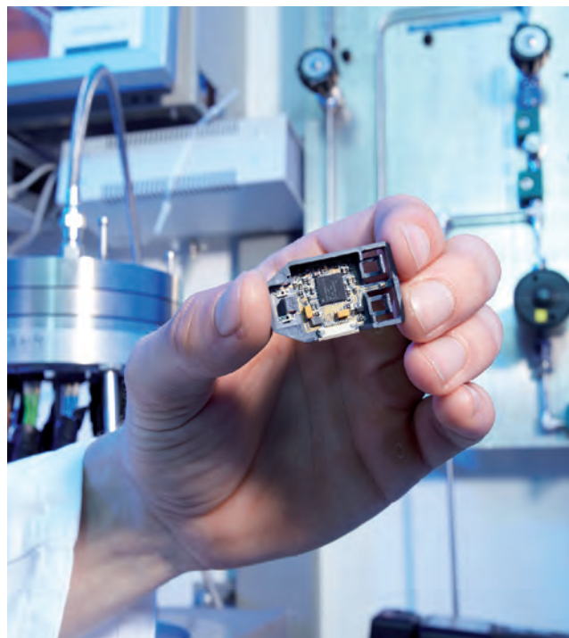
Small, colorimetric and cost-effective: gas sensors, produced in a roll-to-roll process, measure toxic fire gases such as carbon dioxide and nitrogen dioxide.
