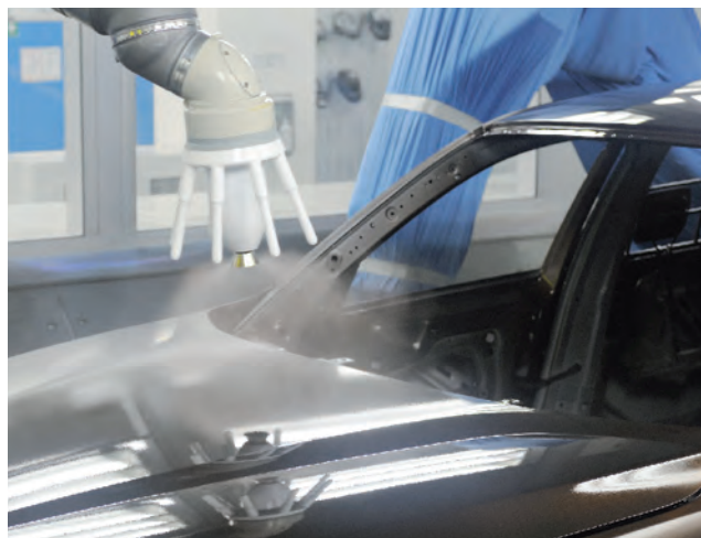
Terahertz waves enable layer thicknesses to be measured without making contact, non-destructively and independently of substrate.
