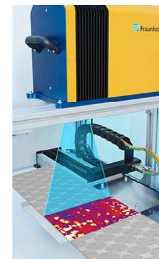
The F-Scanner measures coatings quantitatively using the fluorescence signal of the coating material applied. Evaluation is performed in real-time and thus allows processes to be optimized automatically.
