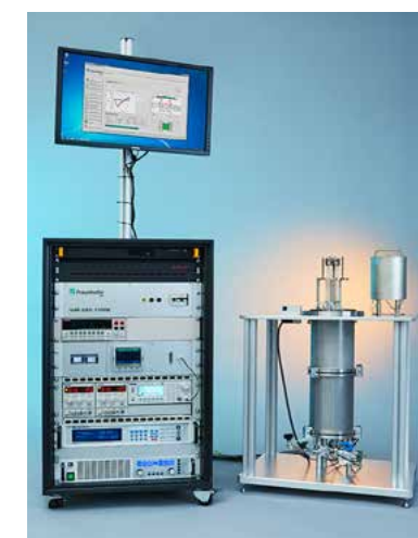
The SRX-vdP measuring system combines the advantages of different measuring methods. The individual methods are already being employed in commercial laboratory devices for materials characterization.
